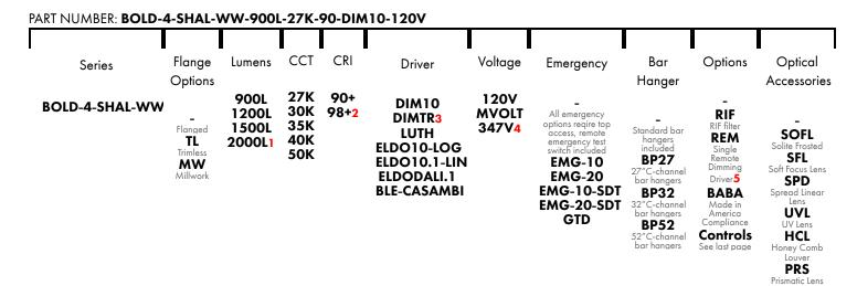
Any fixture can take maximum 2 Optical Accessories 1 The highes lumen will not be compatible with any optical accessories 2 98 + CRI is available only on 27K, 30K and 40K 3 DIMTR is only available with 120V 4 347V is only available with DIM10 5 Remote mount Maximum distance from light fixture to remote power supply is 100' using 14 gauge wire, 50' using 16 gauge wire
