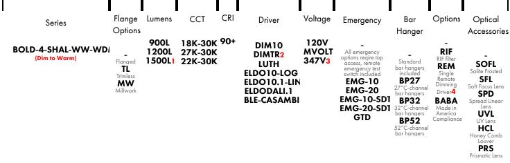
Any fixture can take maximum 2 Optical Accessories 1 The highes lumen will not be compatible with any optical accessories 2 DIMTR is only available with 120V 3 347V is only available with DIM10 4 Remote mount Maximum distance from light fixture to remote power supply is 100' using 14 gauge wire, 50' using 16 gauge wire
